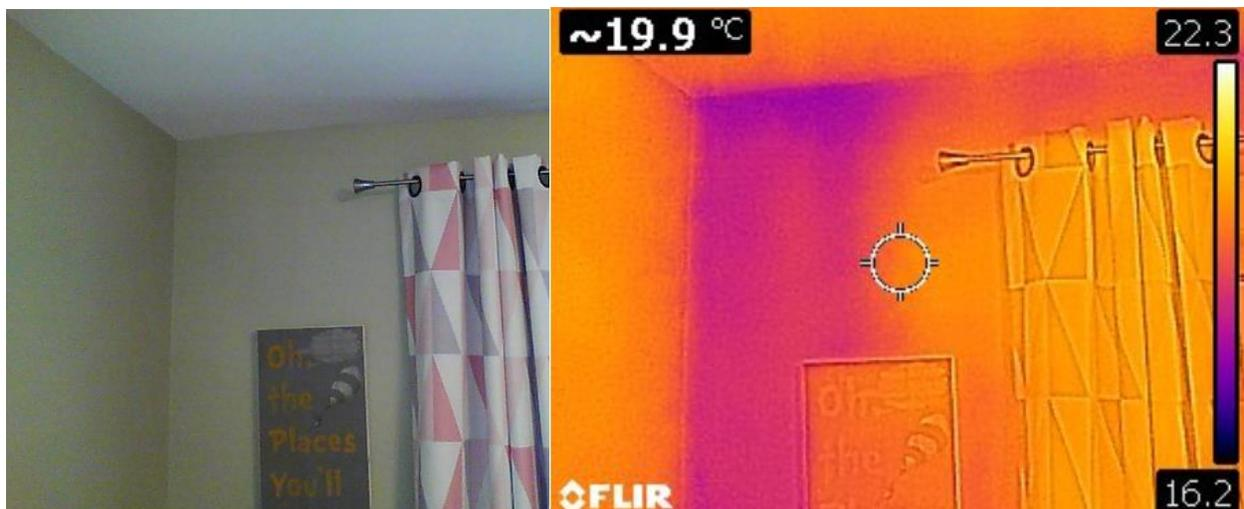
The top left corner of the master bedroom closet (shown in picture and infrared image below) had a small presence of elevated moisture.
