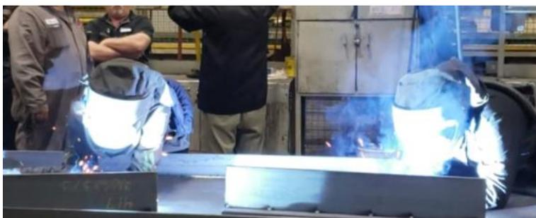
The welder on the left has gun exhaust and the welder on the right does not. Which one looks most like your welders?
