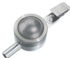
As the occupational exposure limit for wood dust is based on inhalable dust, the samples were collected with SKC Button samplers. These samplers allow only the inhalable fraction of airborne dust to be collected so that the results can be compared directly to the occupational exposure limit for wood dust.
