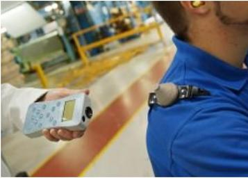
Worker noise monitoring is performed by placing a small noise dosimeter on the worker’s shoulder. There are no wires or boxes – just a small cone that is worn. The dosimeter records the worker’s noise exposure over the course of the day. It doesn’t record the words – only the sound levels in decibels. At the end of the day, the dosimeter is retrieved and the data is downloaded.
