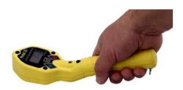
A Ludlum Frisker can be used to look for ionizing radiation such as radioactive contamination in metal from outside Canada
