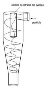
The cyclone filters out the larger particles leaving only the smaller respirable silica particles on which the exposure standard is based. Air passing through the cyclone creates a vortex. Larger particles rub against the inside of the cyclone and fall to the bottom. Finer particles stay airborne and are carried up and into the cassette where they are caught on the filter in the cassette and later analysed at the lab.
