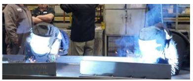
The welder on the left has gun exhaust and the welder on the right does not. Which one looks most like your welders? In light of the magnitude of the exposures, the following actions are recommended:
