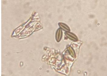
**Left**: Sampling kit includes a high-volume pump, a stand and a mould cassette. **Right**: Four mould spores can be seen in the image taken from the sample. The "cornflakes" in the image are human skin cells.
