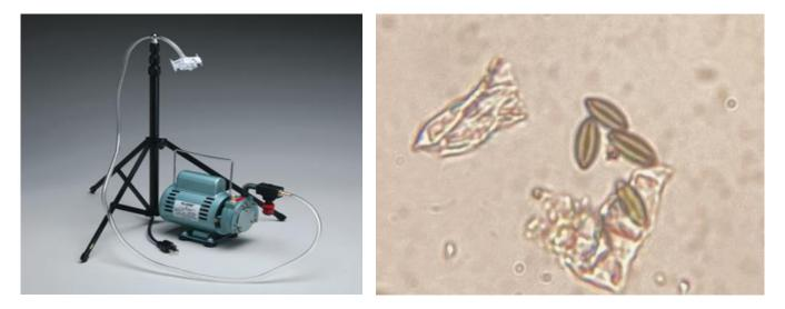
**Left**: Sampling kit includes a high-volume pump, a stand and a mould cassette. **Right**: Four mould spores can be seen in the image taken from the sample. The "cornflakes" in the image are human skin cells.
