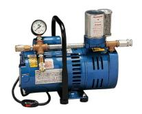
**Left: Ambient Air System:** These smaller units are often seen in autobody shops but can also be seen factories. The units are about the size of a sewing machine and typically operate at 15 PSI or less. These units typically supply air to a single worker but can sometimes serve 2 workers depending on the horsepower of the unit and whether the workers are wearing loose hoods or tight-fitting respirators.
